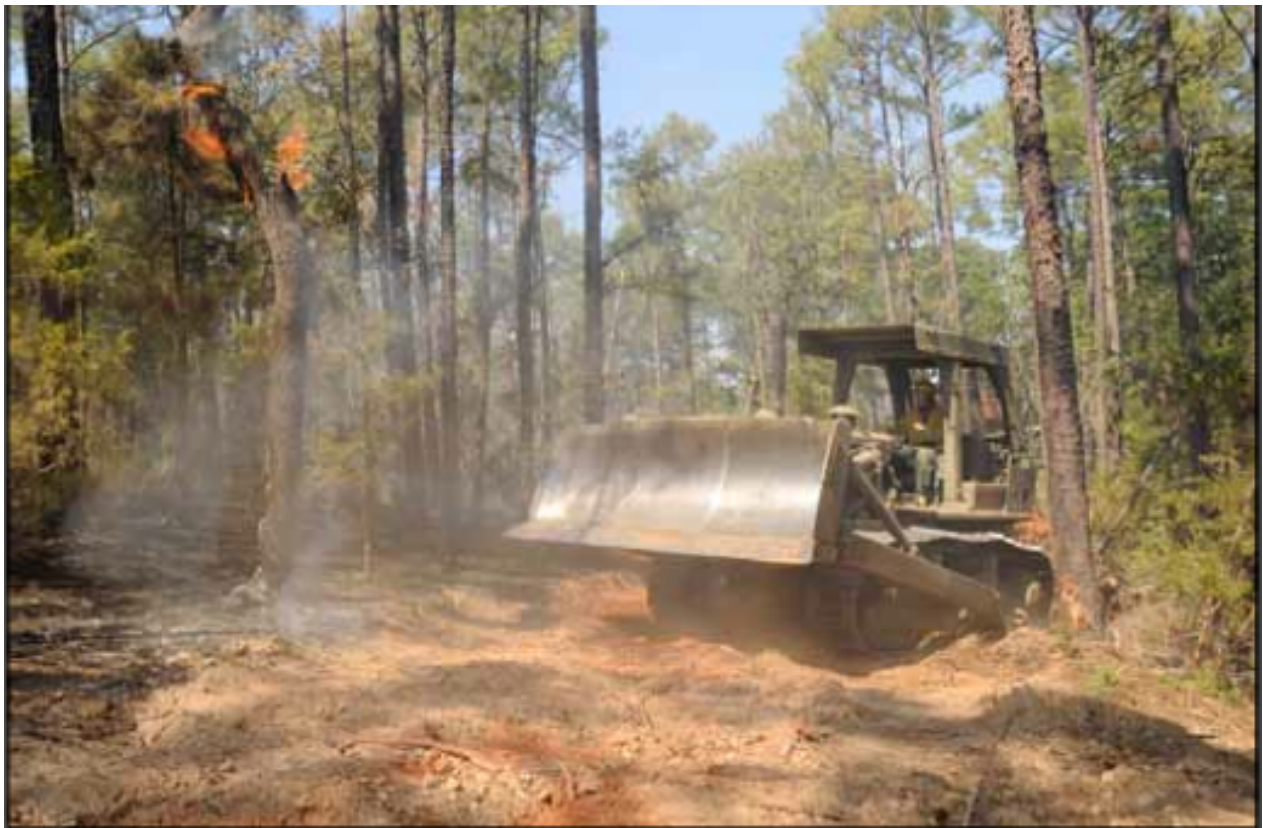
Spc. Brady Burton with the 111th En. Bn., TXARNG, clear trees and brush to create a firebreak during the Bastrop County Complex fire in near Bastrop, Texas.
